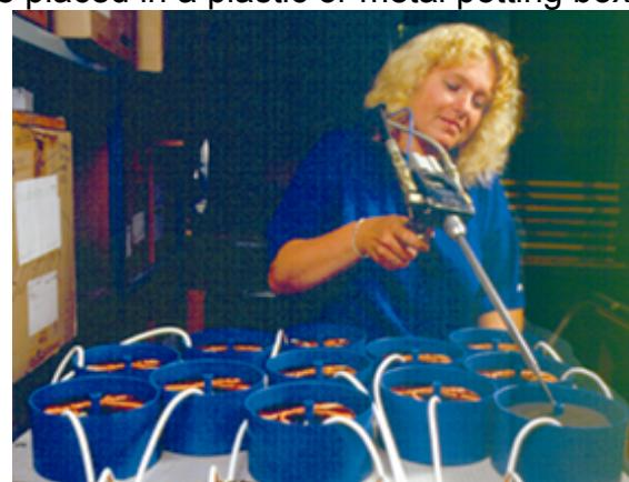
Electrical potting compound is used for protection and insulation
